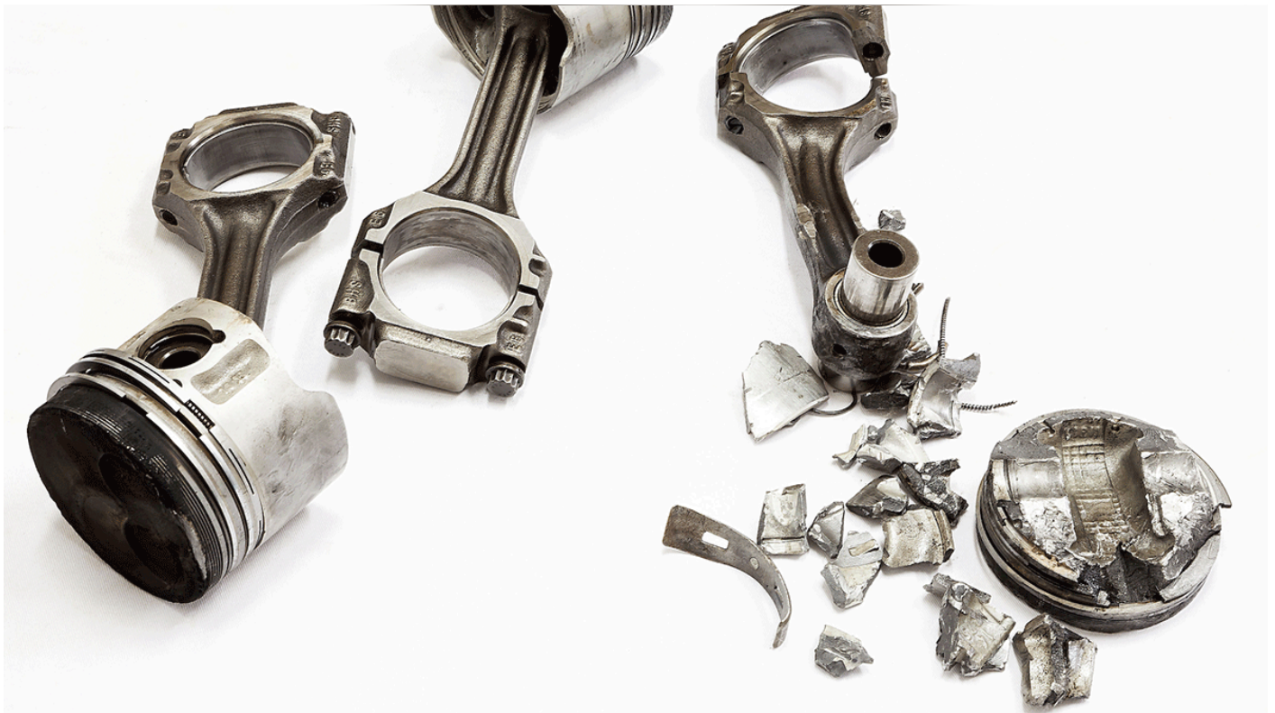
Low-speed pre-ignition (LSPI) is an abnormal combustion event that can ruin pistons.
